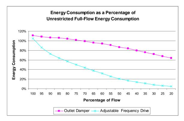
Install high efficiency motors and adjustable frequency drives on the following equipment:
